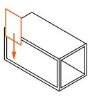
Each Space CUBE steel frame is equipped with special profiles, allowing mounting of light walls, windows, roofing and stairs, terrases and balcony thus modifying space and functions. It is possible to create a single Space CUBE box or demanding Architectural structures consisting of many combined and stacked modules.
